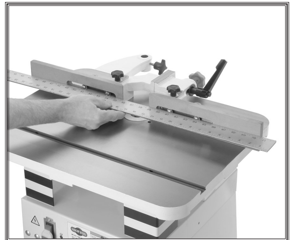
Figure 19. Use straightedge to check fence.
